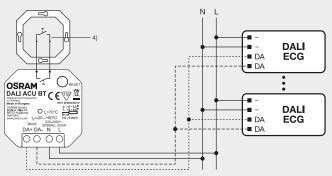
Length of the DALI control cable: up to 300 m Length of the pushbutton cable: up to 50 m
