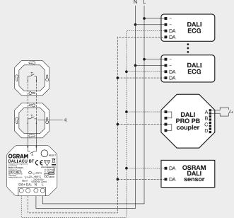
Length of the DALI control cable: up to 300 m Length of the pushbutton cable: up to 50 m
