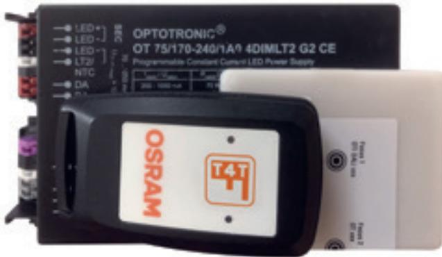
With Feig ECCO Smart, target the NFC antenna of the driver either from the front or the bottom of the scanner.
