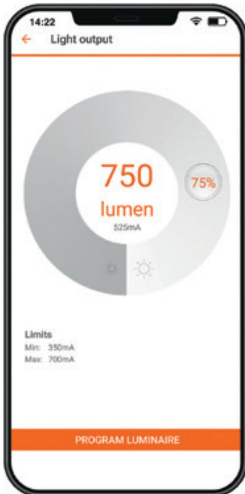
Tapping on the light output value in the middle of the circle enables you to enter an exact value.
