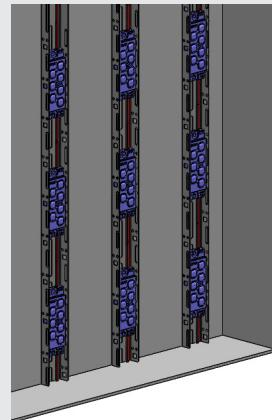
On the back wall of the light box with BackLED® modules
