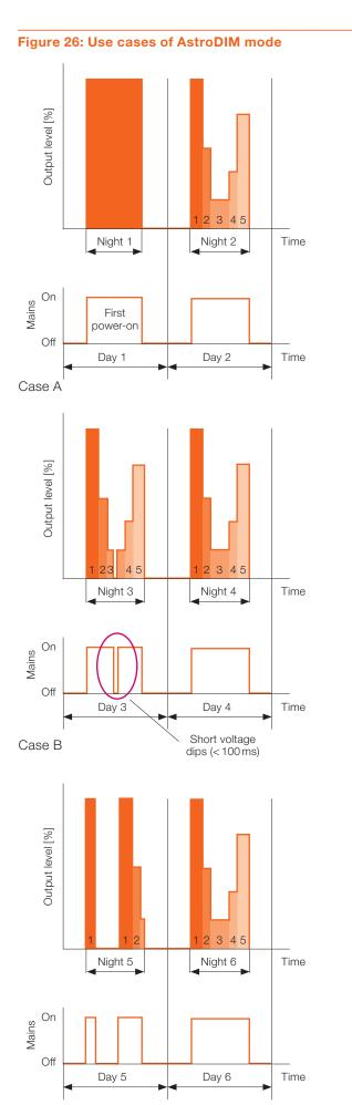
The AstroDIM profile is performed after the first valid on-time.
