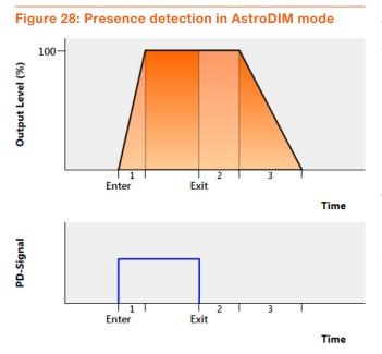
An active signal at the SD(2) port (PD signal) starts the presence detection profile, which is defined by the following four parameters:
