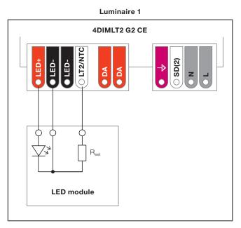
To achieve a more accurate current setting, the second LED- terminal of the LED driver can be used as shown in figure 9. This increases the accuracy by roughly 0.5%.
