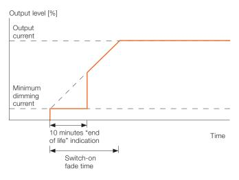
If the switch-on fade time is shorter than 10 minutes, the output current is directly switched to the nominal output level after the "end of life" indication as shown in figure 18.
