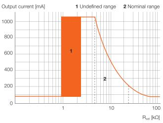
The corresponding output current can be calculated with the following formula within the valid resistor range ( $R_{set} = 4.75-24.9 \, k\Omega$ ):
