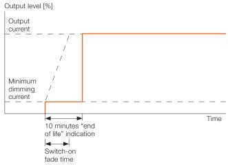
If a switch-on fade time is set, it is overriden by the "end of life" functionality as shown in figure 17. After 10 minutes, the output current is set according to the current switch-on fade time level.
