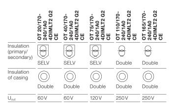
The equipotential pin (EQUI) meets the requirements for double insulation versus the primary side and requirements for basic insulation versus the secondary side (it complies with the requirements of IEC 60598-1 Annex A – "safe to be touched" – in case of insulation fault between all secondary circuits and accessible conductive parts).
