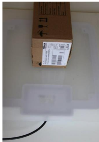
Figure 5: Orientation of the box to antenna ANT310/310
