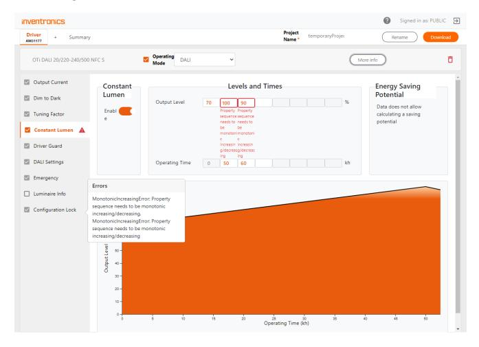
Press the driver tab in the top line to open the driver page. The driver page allows entering all data required by the driver, including project related data. When opening a project from scratch and selecting a driver, data is filled with default settings provided by the device description file from the DD store in the cloud. The default project name can be changed any time by pressing change project name. Press "More info" to read and edit driver and luminaire related data.
