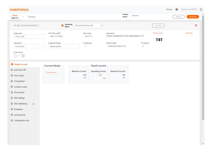
Press "More info" to access additional info on the driver, e.g. GTIN and BaseCode (First 7 digits from IC on the driver label), Serial Number (only available, when reading data from LED drivers), FW version, luminaire image and driver datasheet. Select Driver Count > 1, to enable multiple driver programming via DALI.
