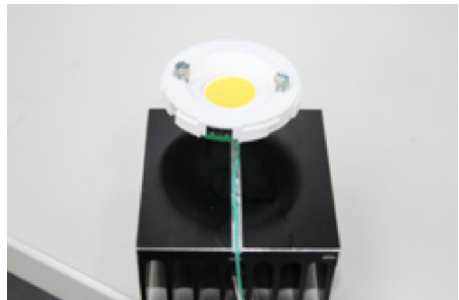
Mounting of a thermocouple by means of a groove
