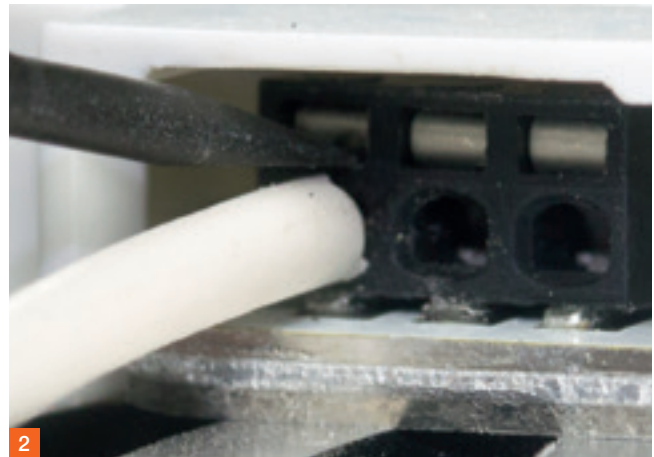
Push in the screwdriver below the release spring
