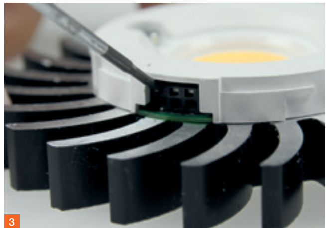
Pull out the wire and afterwards the screwdriver
