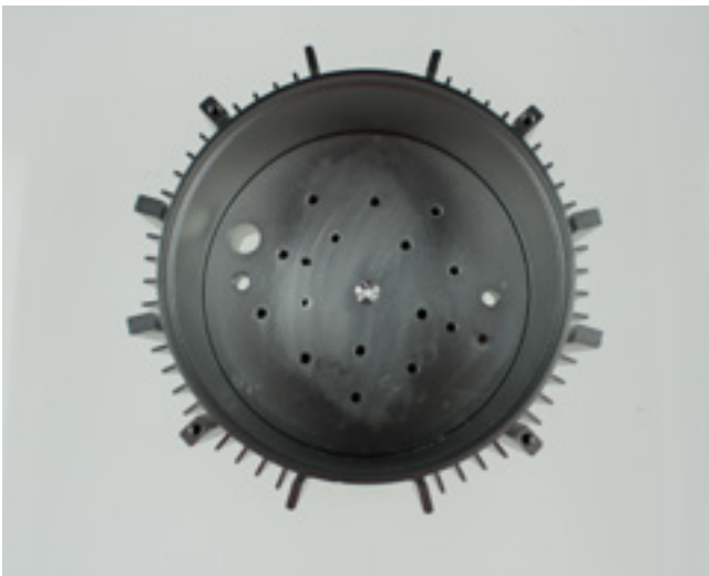
Drill the mounting holes and a hole for the thermocouple
