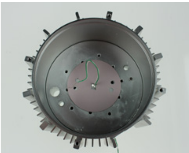
Run the thermocouple through the hole and cut out the TIM
