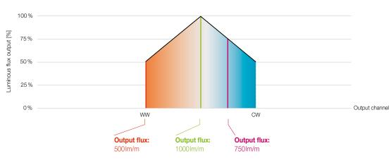
DT6 TW operation: Luminous flux output @ max load / 100 % dimming
