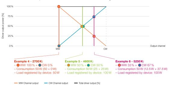
DT8 TW: Power distribution per channel and in total @ max load / 100% dimming
