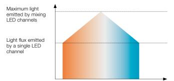
So, if we want to keep the output flux steady while shifting the light color temperatures, we have to use a controller by DT8 which by software restricts the output flux as the one emitted by a single LED color.
