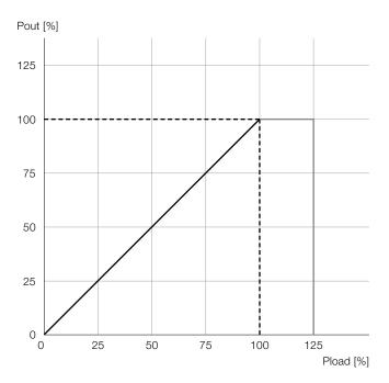
On DALI-controlled systems, in case of an overload situation, the current flow increases, but the system automatically dims the output so the average power remains at 100 % without exceeding this limit.
