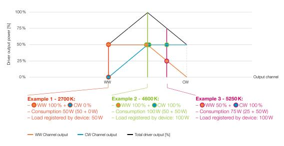
DT6 TW: Power distribution per channel and in total @ max load / 100 % dimming
