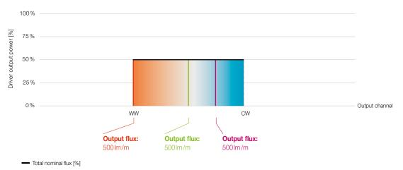
Figure 15: Power consumption of each channel by a TW LED strip with a general DALI DT8 LED driver
