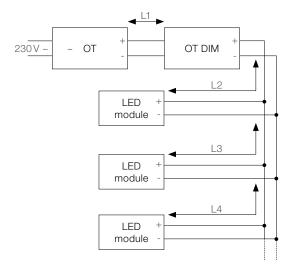
In this example the total length  $L_{total}$  of secondary cables is  $L_{total} = L_1 + L_2 + \ldots \, L_n$
