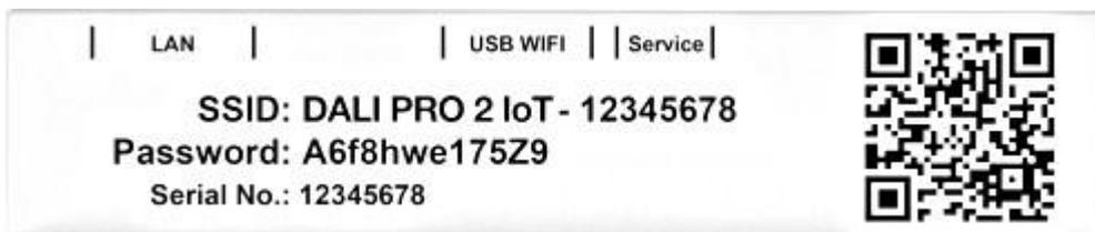
The LED above the button lights up constantly to indicate that the WLAN is ready for use and appears in the list of available WLANs. The network or SSID name, which is also printed on the device, begins with "DALIPro2-" and contains the serial number of the device:
