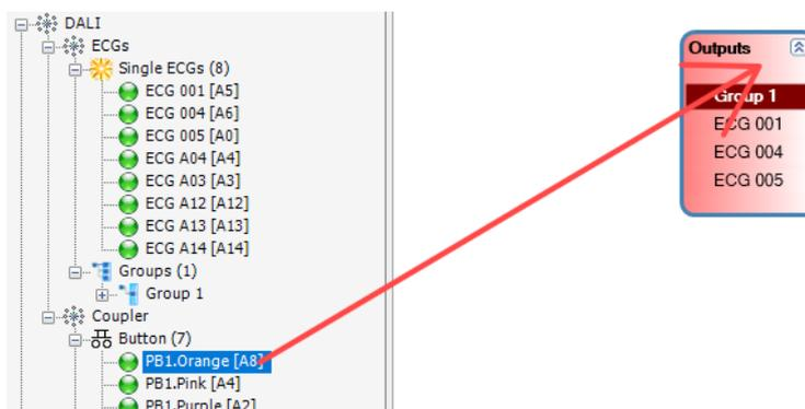
The connection fixes the devices in the current zone. If no zone exists, a new zone is automatically created.
