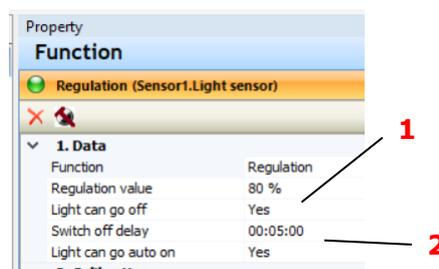
It is also possible to switch the light on again automatically if the brightness in the room falls below the set value by setting the "Light can go auto on" property to "Yes" (2).
