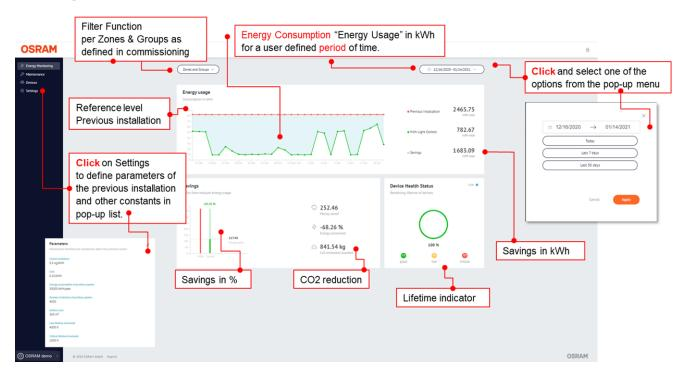
Step 5 **View the Dashboard (Maintenance)** Indicator to show how many of **OSRAM** the installed drivers are on-line Color coding for remaining lifetime Exploded view Mo devices <1000 h 3109 10.36 100 60 Devices >4000 h zone Exploded view group group Power indication group Click on a zone Zones Groups within a zone a displayed as well
