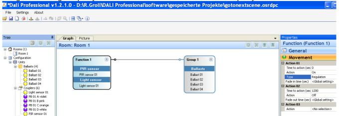
For practical reasons it is always an advantage if there are some additional pushbuttons to have a chance for manual control – e.g. if PIR sensor gets defect / dirty / shielded ...
