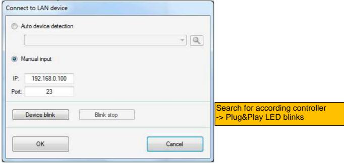
Alternatively automatic IP setting can be started with DHCP = Yes in controller settings
